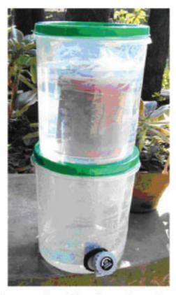
The pottery candle system shown above gives 2.0 to 3.0 liters of filtered water per hour. The system is very effective, acceptable to users and low priced. These can be made almost anywhere, using local resources.
